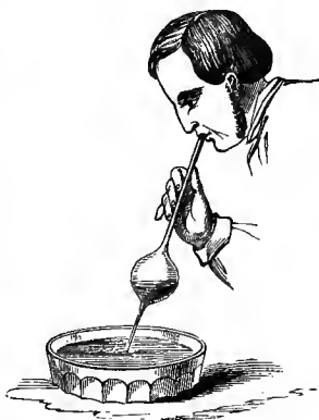
PIPETTE TO DRAW OFF SMALL PORTIONS OF OTTO FROM WATER.
